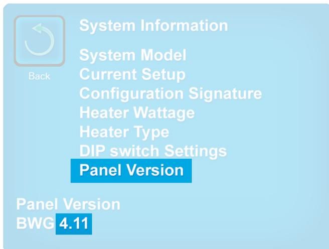
Select "Panel Version." The panel software version appears at the bottom of the screen. In this example it's 4.11.
