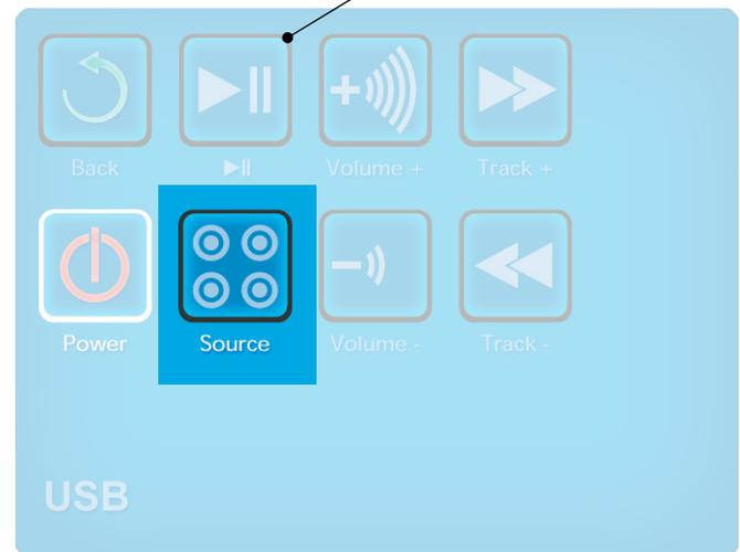
The "Source" button switches between Bluetooth, USB, and Line In input modes.
